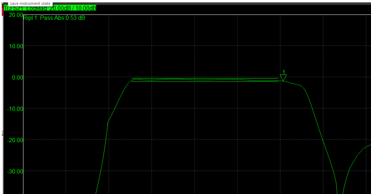
Figure 21 Ripple test measuring the ripple of the passband in a passband filter.
